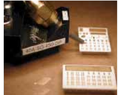
Calibration with impedance standard substrate
