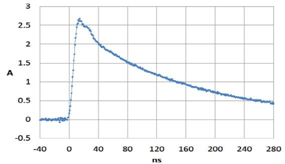
Built-in current measurement of 4kV HBM pulse
