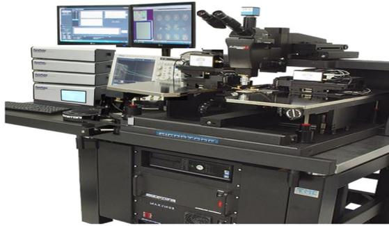
PurePulse HBM Flying Probe automatic test system
